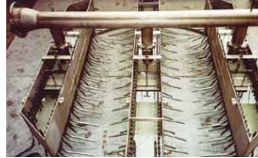
UniFlo® Acid Distributor baffle and gate assembly
